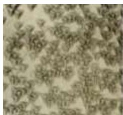
Hillocks on a GaAs (111)-surface grown from the gas phase via metalorganic chemical vapour deposition (MOCVD).
